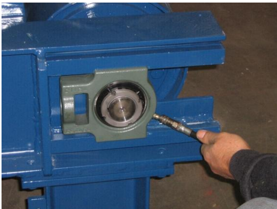
Figure 15 – How to grease the pair of rear bearings.
