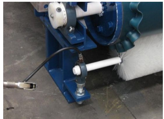
Figure 16 – How to grease the bearings of brush (if any installed).
