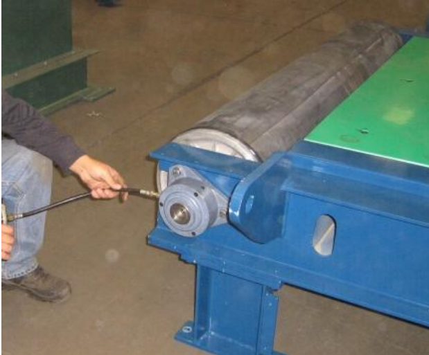
Figure 13 – How to grease the pair of external bearings.
