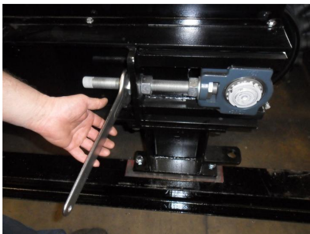
Fig. 17 - Belt adjustment.
